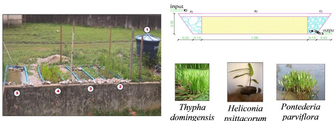
1 Reservoir; 2 CW planted with Thypha; 3 CW planted with Heliconia; 4 CW with Pontederia; and 5 CW not planted.
