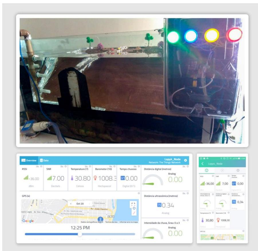
**Figure 5.** Laboratory environment with sensors coupled in a flood scenario and visualization on web and mobile dashboards.
