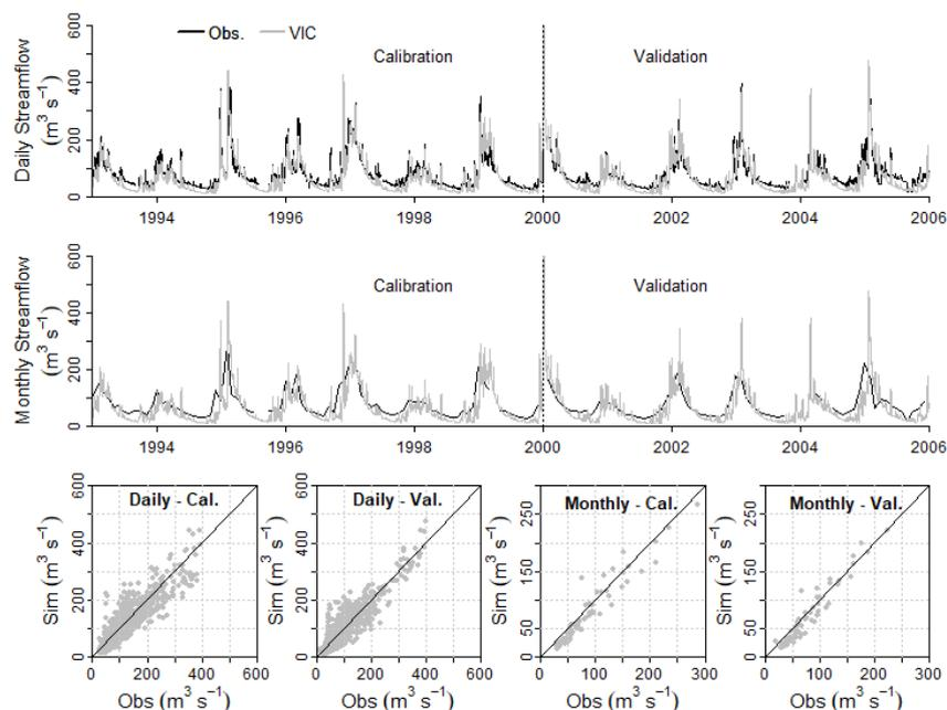
**Figure 2.** Observed and simulated daily and monthly discharges during calibration (1993-1999) and validation (2000-2005) periods.
