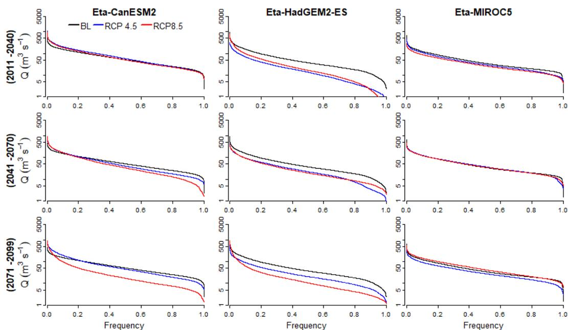
**Figure 6.** Flow Duration Curve (FDC) of daily discharge ( $Q$ ) simulated by VIC using data of baseline (BL) and future scenarios (RCP4.5 and RCP8.5) projected by the RCMs (Eta-CanESM2, Eta-HadGEM2-ES and Eta-MIROC5).
