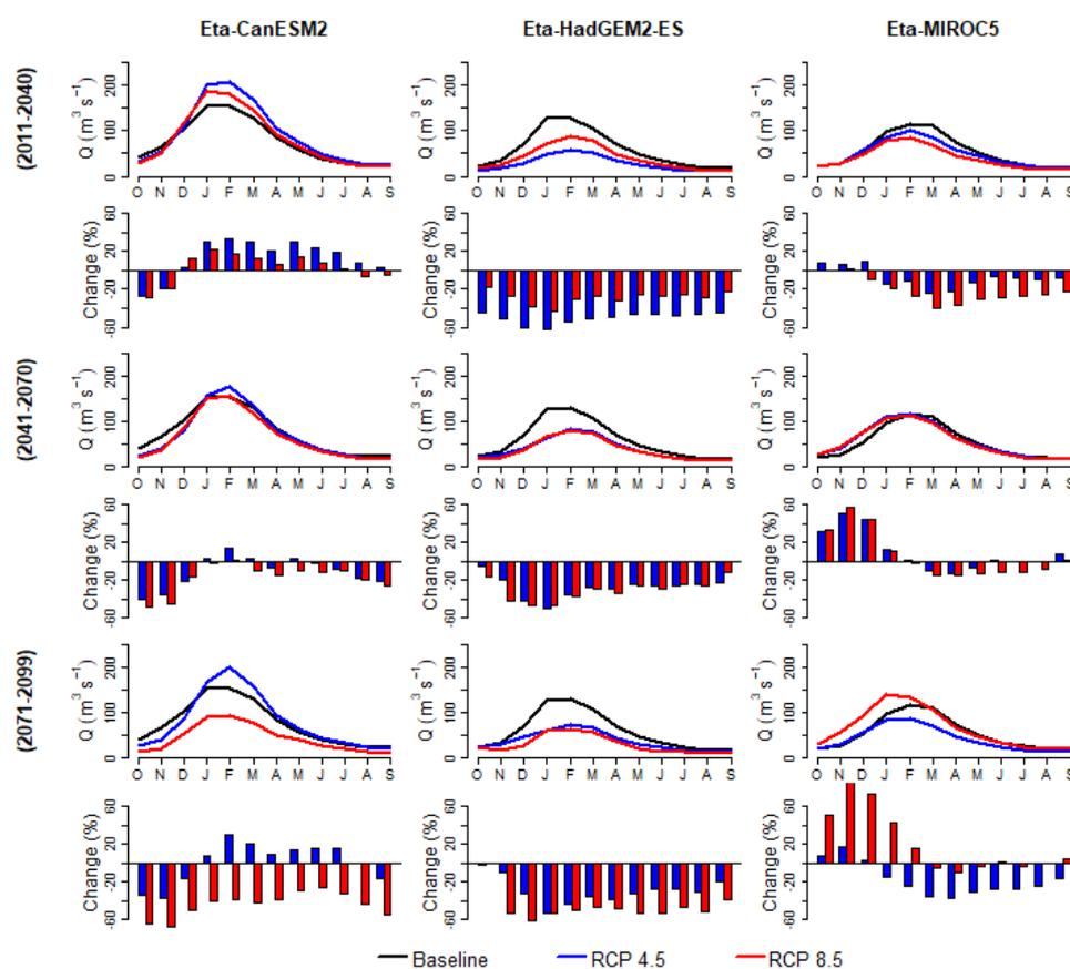
**Figure 4.** Mean monthly discharge (Q) simulated by the VIC model forced by RCMs Eta-CanESM2, Eta-HadGEM2-ES, and Eta-MIROC5 for the three time-slices (2011–2040, 2041–2070, and 2071–2099) under RCP4.5 (blue) and RCP8.5 (red), and changes (%) of both scenarios relative to the baseline period (1961–2005).
