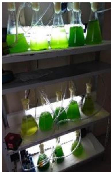
**Figure 1.** Photobioreactors in a controlled environment.
