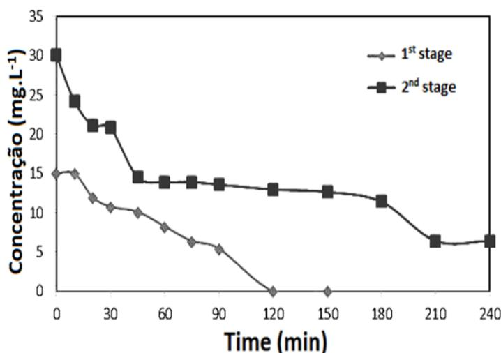
**Figure 2.** Degradation profiles of 17 $\alpha$ -ethynylestradiol at initial concentrations of 15mg L<sup>-1</sup>(◆) and 30mg L<sup>-1</sup>(■) in the presence of UV light and 0.02% TiO<sub>2</sub> (pH 7.0).
