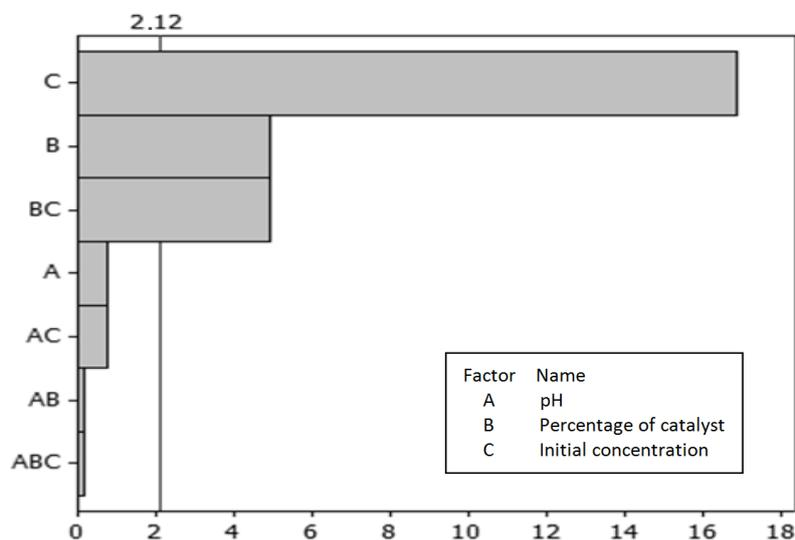
**Figure 1.** Pareto diagram showing the magnitude of the effects of the reaction parameters (**A**, pH; **B**,  $\text{TiO}_2$  concentration; **C**, initial concentration of  $17\alpha$ -ethynylestradiol) on the degradation of  $17\alpha$ -ethynylestradiol ( $p = 0,05$ ).
