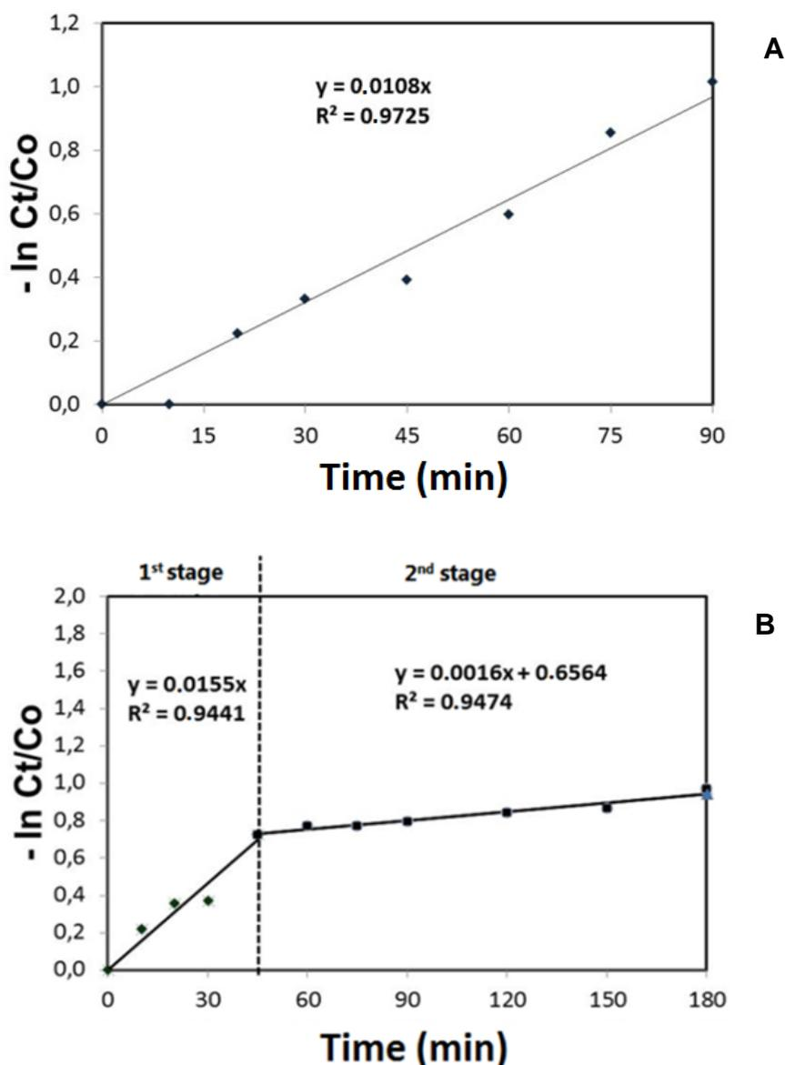
**Figure 3.** Rates of degradation of 17 $\alpha$ -ethynylestradiol at initial concentrations of (A) 15 mg L<sup>-1</sup> and (B) 30 mg L<sup>-1</sup> in the presence of UV light and 0.02% TiO<sub>2</sub> (pH 7.0) (p=0,05).
